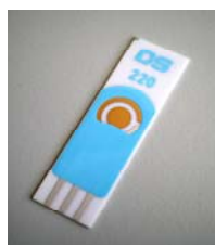
220AT High temperature curing ink, WE 4mm
