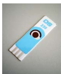
220BT Low temperature curing ink, WE 4mm
