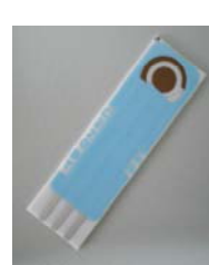
C220BT Low temperature curing ink, WE 4mm. Work in solution
