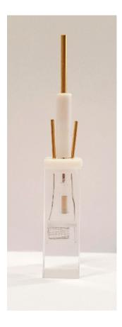
The cell includes also the platinum grid working electrode, the platinum counter and a silver/silver chloride reference electrode.
