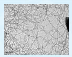
**Dropsens** Single- and Multi-Walled Nanotubes are produced through **Chemical Vapour Deposition (CVD)**. Also functionalised with -COOH and -NH<sub>2</sub> groups. They are suitable for mechanical and electrical applications.
