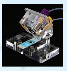
It can be used with all DropSens Screen-Printed Electrodes with the sensing part in the middle of the strip.
