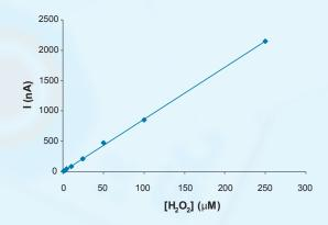
Calibration curve for hydrogen peroxide (in a 0.1 M phosphate buffer pH 7.2) from 1·10<sup>-6</sup> M to 2.5·10<sup>-4</sup> M in a FIA system (ref. FIASYSTEM using our Screen-printed Co-Phthalocyanine/Carbon electrodes. E<sub>det</sub> +0.4 V; Flow rate 2.2 ml/min
