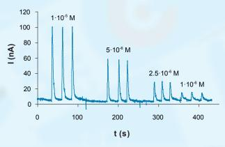
Amperometric detection of hydrogen peroxide in a flow injection analysis system with our easy to use flow cell (ref. FLWCL). The amperometric responses for decreasing H<sub>2</sub>O<sub>2</sub> concentrations at a ref. 410 electrode show neither fouling nor memory effects. E<sub>det</sub> +0.4 V; Flow rate 2.2 ml/min; Flow carrier 0.1 M phosphate buffer, pH 7.2
